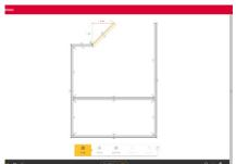
The first step is to create your floor plan, select the formwork system and enter some basic variables of the project.
